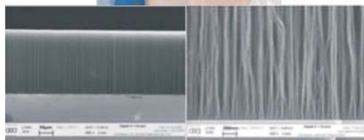
Figure 5. Dense forest of Small diameter MWCNT from left to right: a) Patterned layer on a 200mm layer b) 50µm high forest on conductive layer of TiN c) close view of the material with individual CNT making bundles of 60nm of diameter (courtesy of CEA-LITEN).
