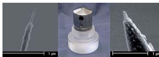
Figure 10. Left, electron micrograph of a single CNT grown on a tungsten tip. Note that the growth is aligned with the tungsten axis. Centre, a tungsten tip mounted in a suppressor module. Right, a CNT grown on a tungsten already mounted in the suppressor in situ.
