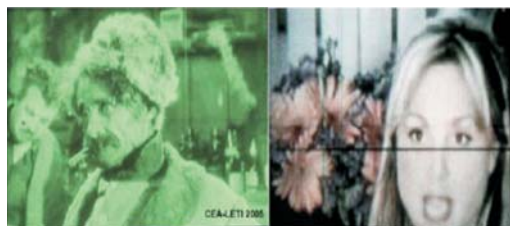
Figure 7. Two stages of development of CNT FED at CEA. On the left: monochrome display with 350 μm pixels, on the right: color video display with 600 μm pixels. On these display the non uniformity from pixel to pixel is 5% while it is 3% with LCD displays and 2% for CRT (courtesy of CEA-LITEN).
